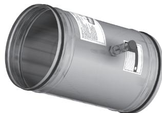
The Barcol-Air constant-air-volume-terminals, type NR / NT are factory pre-set on the desired air volume. The air volume can be changed within the ranges of the unit and read on a scale. Adjustment goes manually by Allen key.
