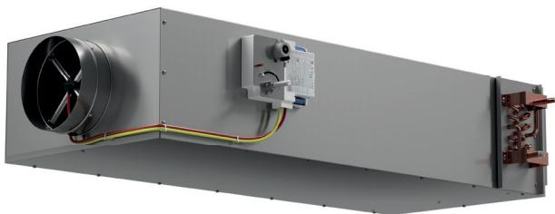
using at least two support brackets (DIN-rail or L-profile), with anti-vibration rubber under the terminal. Each of these brackets shall be fixed with two threaded rods to the ceiling slab above.
